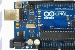
Gambar 4. Papan Arduino Uno R3
