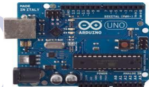
Gambar 2. Board Arduino Uno R3 (Sumber : datasheet,2017)
