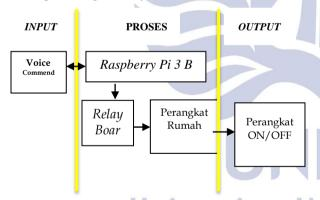
Gambar 4. Blok Diagram Sistem (Sumber: Data Primer, 2019)
