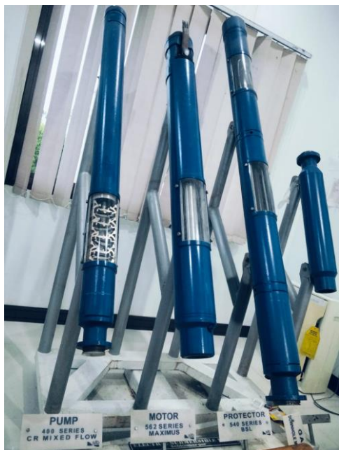
Gambar 1 Foto Komponen Fisik ESP (Pump 400 Series, Motor 562 Series Maximus, Protector 540 Series, Gas Separator) — Dokumentasi Lapangan
