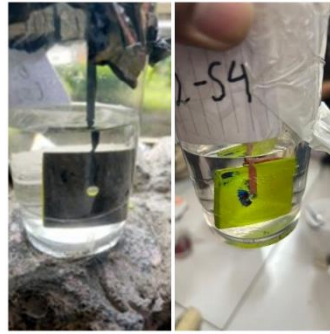
Figure 4. Corrosion Test Samples/Plates
