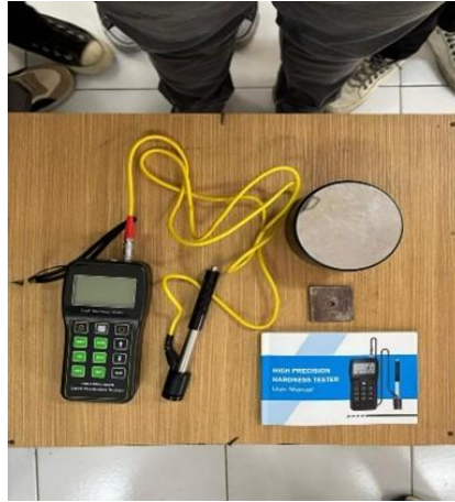
Figure 2. Hardness Testing Device
