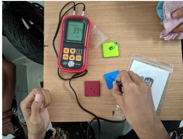
Figure 3. Thickness Testing Process
