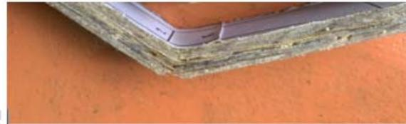
Gambar 7. Penampang Patahan Bending Varian bambu Acak
