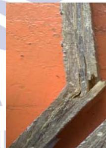
Gambar 8. Penampang Patahan Bending Varian bambu Anyam
