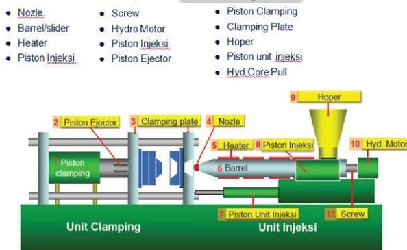
Gambar 2. Gambar Mesin Injection Molding (Sumber :Dokumentasi Pribadi)
