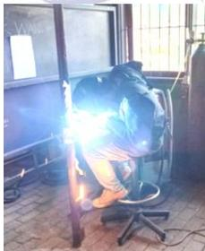
Gambar 4. Proses pengelasan fcaw
