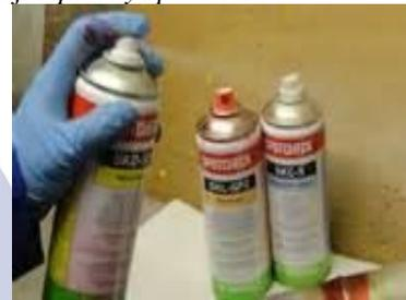
Gambar 5. *Liquid dye penetrant test*
