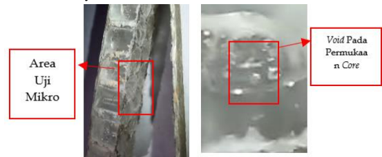
Gambar 5. Hasil Uji Mikro Core Honeycomb
