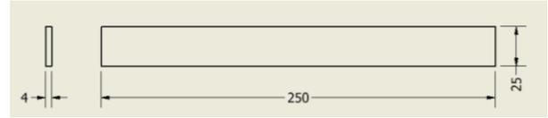
**Gambar 2.** Dimensi Spesimen uji tarik ASTM D3039
