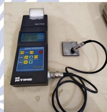
**Gambar 4.** Alat Coating Thickness Gauge.
