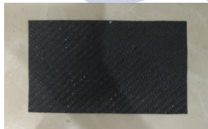
Gambar 8. Hasil Composite Carbon Fiber
