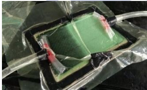
Gambar 7. Proses Laminasi Resin
