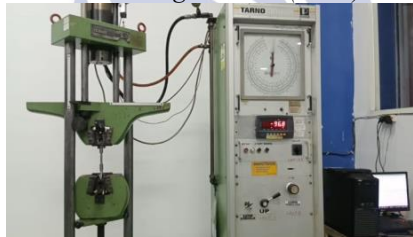
Gambar 4. Universal Testing Machine
