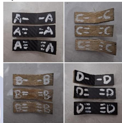
Gambar 8 Material Impact Sesudah Diuji
