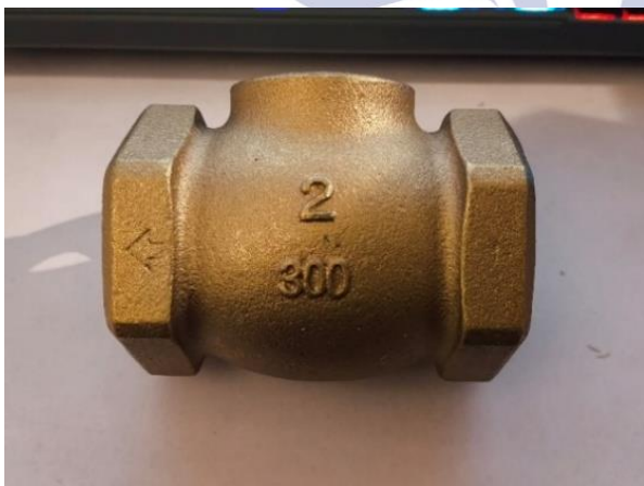
Gambar 6. Hasil Pengecoran Globe valve 2 Inchi
