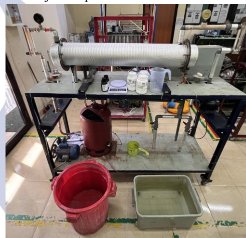
Gambar 6. Alat shell and tube heat exchanger berbaffle heliks hasil rancang bangun
