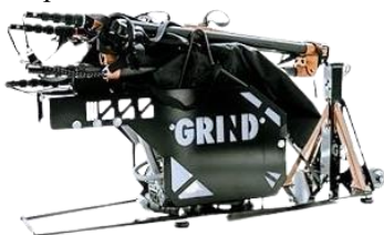
Gambar 1 Mesin Basketball Launcher Berbasis Penggerak Sistem Pneumatik
