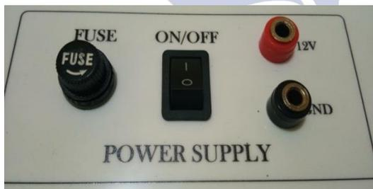
Gambar 4. *Block Power Supply*
