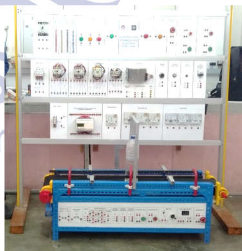
Gambar 3 Trainer Programmable Logic Controller dan Conveyor Pengisian Botol Air Mineral
