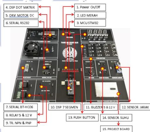
**Gambar 6** Bagian Trainer Mikrokontroler STM32
