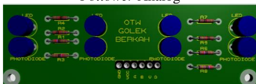
Gambar 2. Desain Hardwere Sensor Trainer Robot Line Follower Analog
