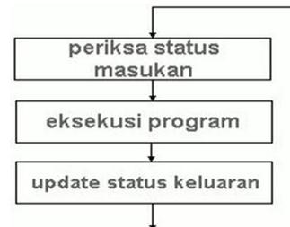
**Gambar 2. Proses scanning program PLC**
