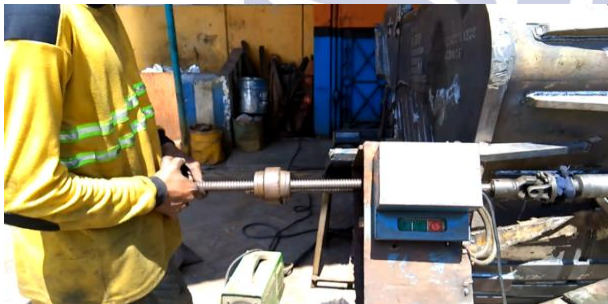
Gambar 1. Pengoperasian Manual Mesin Line Boring di PT SMS
