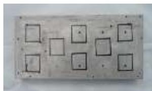
Gambar 10. Penandaan Pada *Heat Sink* Sisi Dingin Dan *Heat Sink* Sisi Panas
