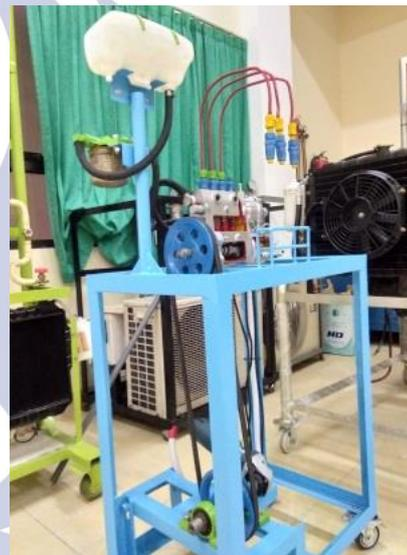
Gambarr 11. Hasil Jadi Trainer Desain Engine Cutting Bosch Pump Tipe In-Line 4 Silinder
