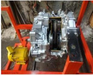
Gambar 10. *Trainer* Transmisi Otomatis Tipe CVT
