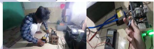
Gambar 8. Proses Pengujian Sistem Kontrol Trafo MOT (Microwave Oven Transformator)
