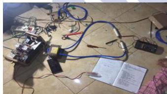
Gambar 9. Proses pengujian Trafo MOT (Microwave Oven Transformator)
