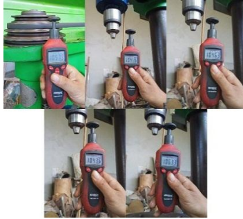
Gambar 7. Pengukuran Tachometer Speed Pulley 2
