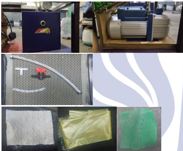
Gambar 11 Tabung Reservoir, Vacuum, Infusion Tube, Spiral Tube, T Connector, Peel Ply, Vacuum Bagging, Infusion Mash
