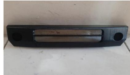
Gambar 5. *Moulding* Positif *3d print*
