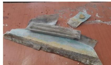
**Gambar 14.** Proses Pelepasan Bumper Dari Moulding Negatif
