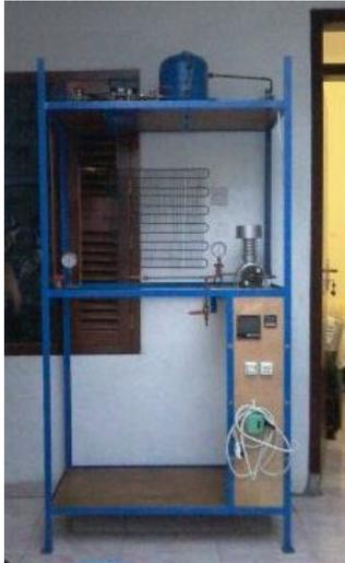
Gambar 7. Rancang bangun alat pengujian efisiensi *wire and tube heat exchanger*
