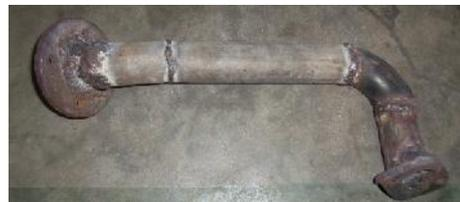
Gambar 12. *Front pipe* modifikasi *diesel engine stand* Isuzu C190
