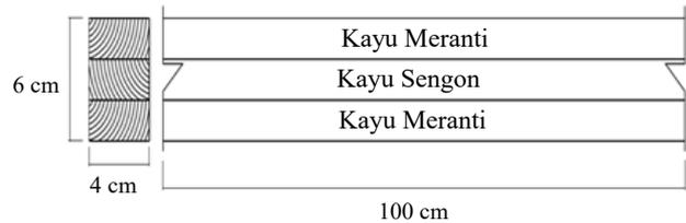
**Gambar 3.** Prototype Benda Uji
