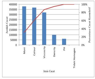
Gambar 2. Diagram Pareto Defect Cat Water Based
