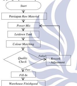
Gambar 1. Flow Chart Proses Produksi Cat Water Based
