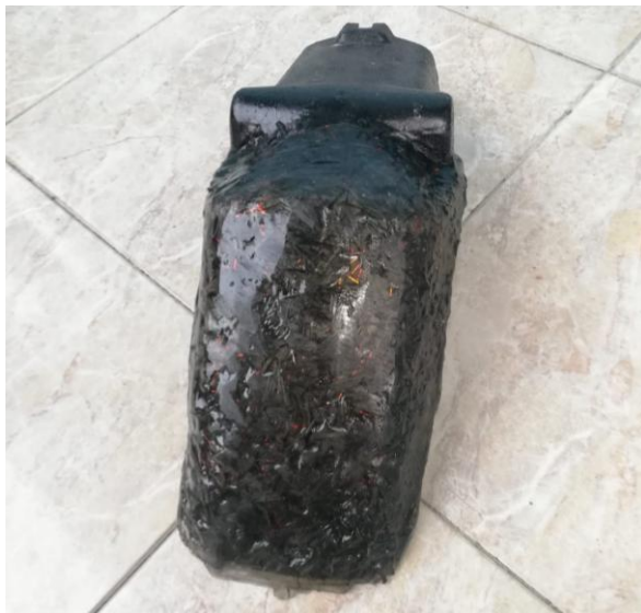
Gambar 27. Skinning Carbon Forged diatas Rear Fender (Sumber: Dok. Perupa 2026)
