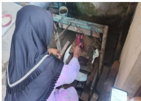
Figure 1. The Pressing Process of Tofu Pulp to Remove Excess Water
