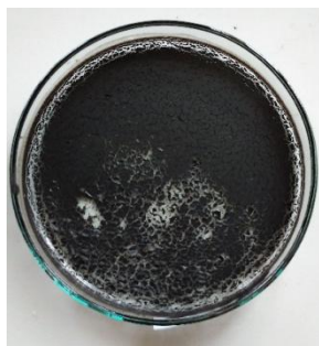
Gambar 1. Hasil sintesis graphene oxide
