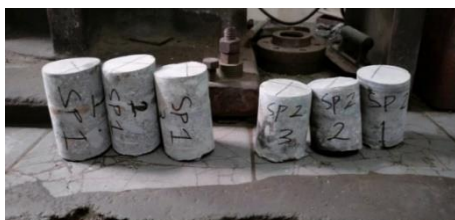
Gambar 2. Sampel Beton Inti ( Core Drill Samples )
