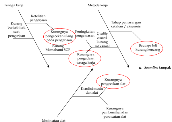
Gambar 6. Diagram Fishbone Cacat Retak
