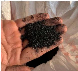
Gambar 1. *Copper Slag*
